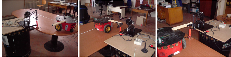
Fig. 3. A mobile robot is used to excite the MHI with a ramp signal: (left) the mobile robot is accelerated to reach V_R velocity; (middle) the mobile robot comes into contact with the MHI end effector; (right) the MHI end effector starts moving.
