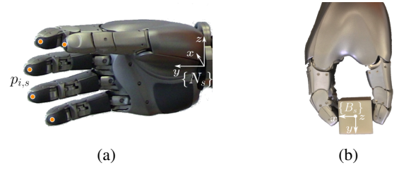
Fig. 4: The slave sub-system setup. (a) A DLR-HIT Hand II with the contact points p_{i,s} ( i = 1, \dots, nc_s ) expressed with respect to the reference frame \{N_s\} . (b) The real cube with its own reference frame \{B_s\} .
