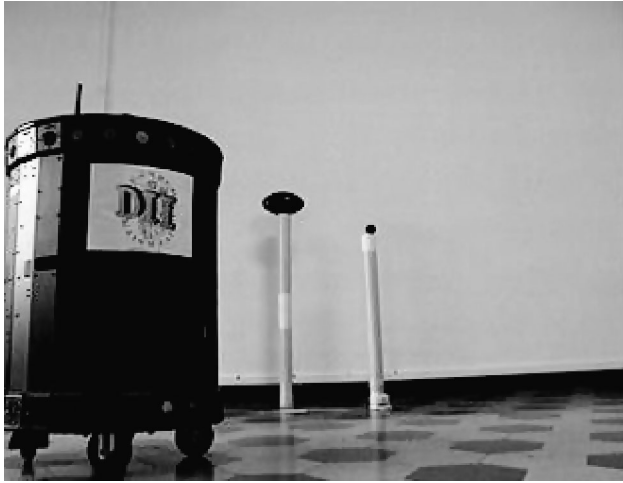
Figure 15. The experimental setup consisting of the camera-robot and two objects with no special image features other than their apparent contours.
