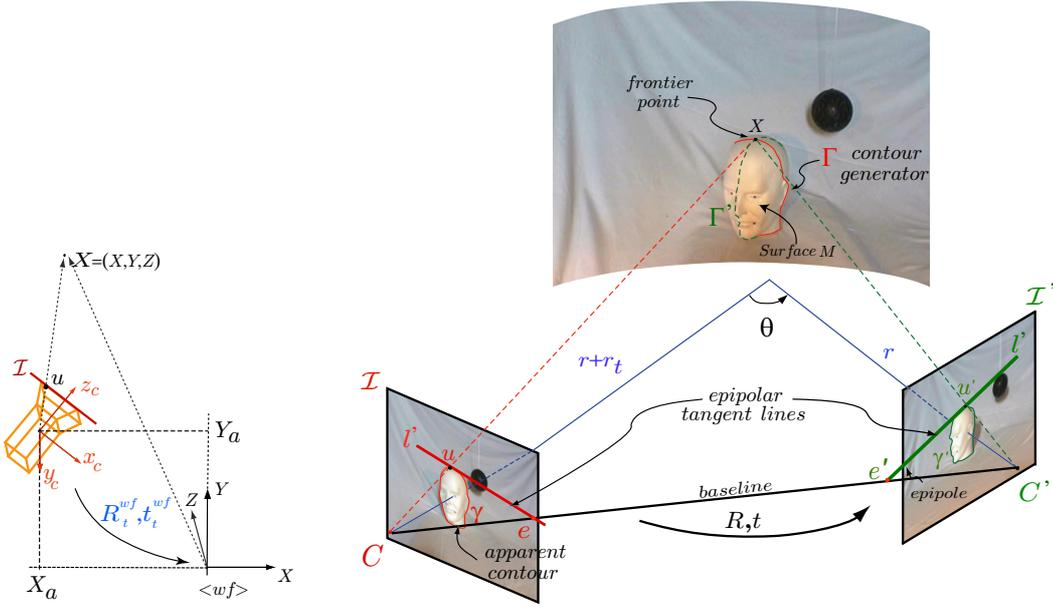
Figure 1: (a) Mobile robot reference frame with pin-hole camera mounted on; (b) Basic epipolar geometry notation.
