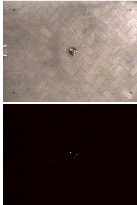
Fig. 4. Actual and filtered images used to detect the robot.
