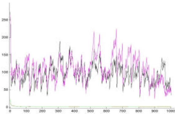
Figure 9: Worst case error bounds for the set-membership tracking (black, x axis; violet, y axis) and 99% confidence intervals estimated by the EKF through the covariance matrix (green, x axis; red, y axis - they overlap in such a way to be almost undistinguishable). X-axis in the figure is in sampling intervals, Y-axis is in meters
