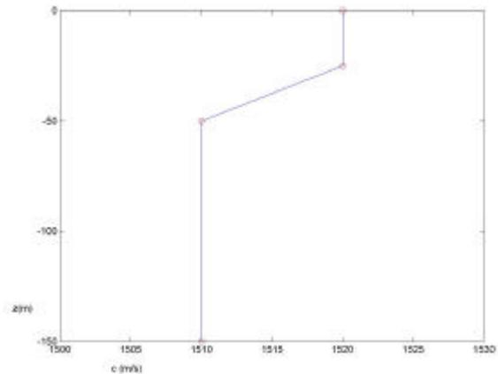
Figure 5: sound speed profile used to generate the data of Figures 6-7. The profile is typical of summer conditions in shallow water. Water depth is 150m.
