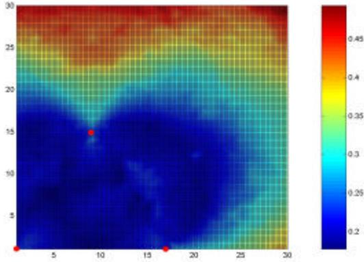
Figure 7: Color-coded average worst case error over the admissible region in the case of Gaussian distributed measurement error, summer conditions. The error chromatic scale is in Km. Buoy locations are the red circles. Scales on the  $x$  and  $y$  axis are in Km
