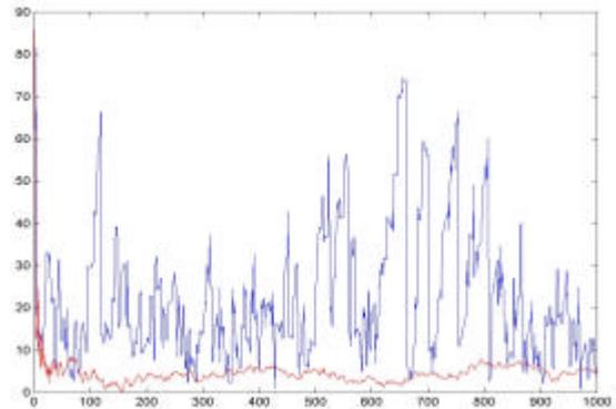
Figure 8: Error as a function of sampling instant along the path for both tracking algorithms. X-scale is in sampling intervals, Y-scale is in meters. The blue line is the error of the set-membership tracking algorithm, the red line is the error of the EKF tracking.
