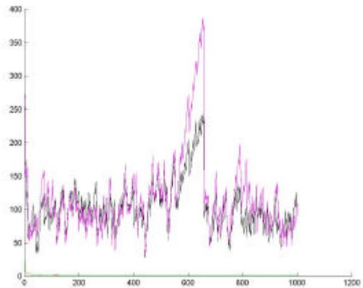
Figure 11: Worst case error bounds for the set-membership tracking (black, x axis; violet, y axis) and 99% confidence intervals estimated by the EKF through the covariance matrix (green, x axis; red, y axis both included in the interval between 0 and 10 m/s, but for the initialization transient). X-axis in the figure is in sampling intervals, Y-axis is in meters
