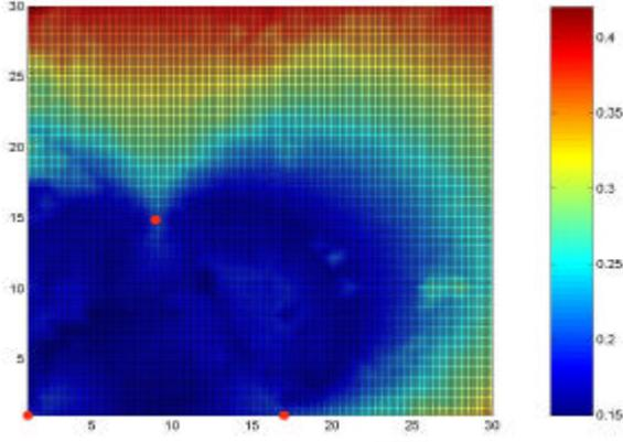
Figure 6: Color-coded average worst case error over the admissible region in the case of uniformly distributed measurement error, summer conditions. The error chromatic scale is in Km. Buoy locations are the red circles. Scales on the  $x$  and  $y$  axis are in Km
