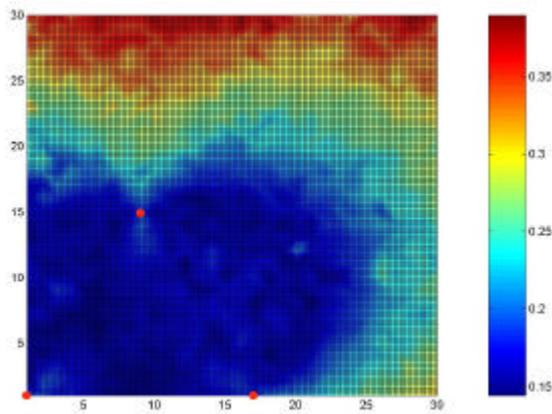
Figure 4: Color-coded average worst case error over the admissible region in the case of Gaussian distributed measurement error, constant sound speed profile. The error chromatic scale is in Km. Buoy locations are the red circles. Scales on the  $x$  and  $y$  axis are in Km.
