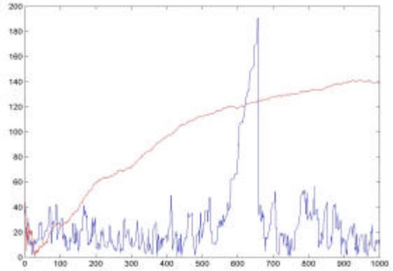
Figure 10: Error as a function of sampling instant along the path for both tracking algorithms. X-scale is in sampling intervals, Y-scale is in meters. The blue line is the error of the set-membership tracking algorithm, the red line is the error of the EKF tracking.
