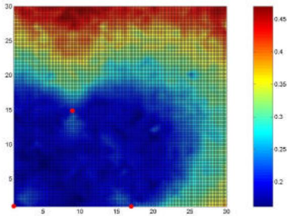
Figure 3: Color-coded average worst case error over the admissible region in the case of uniformly distributed measurement error, constant sound speed profile. The error chromatic scale is in Km. Buoy locations are the red circles. Scales on the  $x$  and  $y$  axis are in Km
