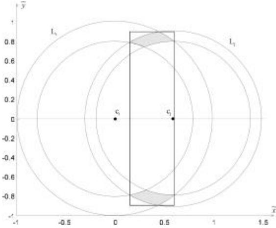
Figure 2: intersection between two spherical caps  $L_i, L_j$  (planar view); the admissible regions for the vehicles are the gray shaded regions. The rectangle represents the box of minimal volume containing the admissible region. The coordinate system has an axis oriented along the line through the buoys  $i, j$  (the centers of the spherical caps).
