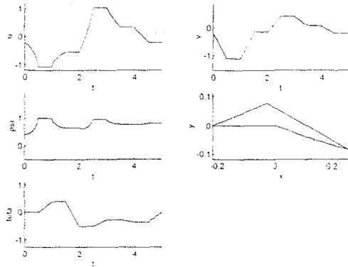
Figure 4: Path from  $\mathbf{x}_0 = [0, 0, -\frac{\pi}{8}, -\frac{\pi}{8}, \frac{\pi}{8}, 0]$  to  $\mathbf{x}_1 = [0, 0, -\frac{\pi}{8}, -\frac{\pi}{8}, \frac{\pi}{4}, 0]$ . The plot in  $x - y$  coordinates describes the path followed by the vehicle in the plane.
