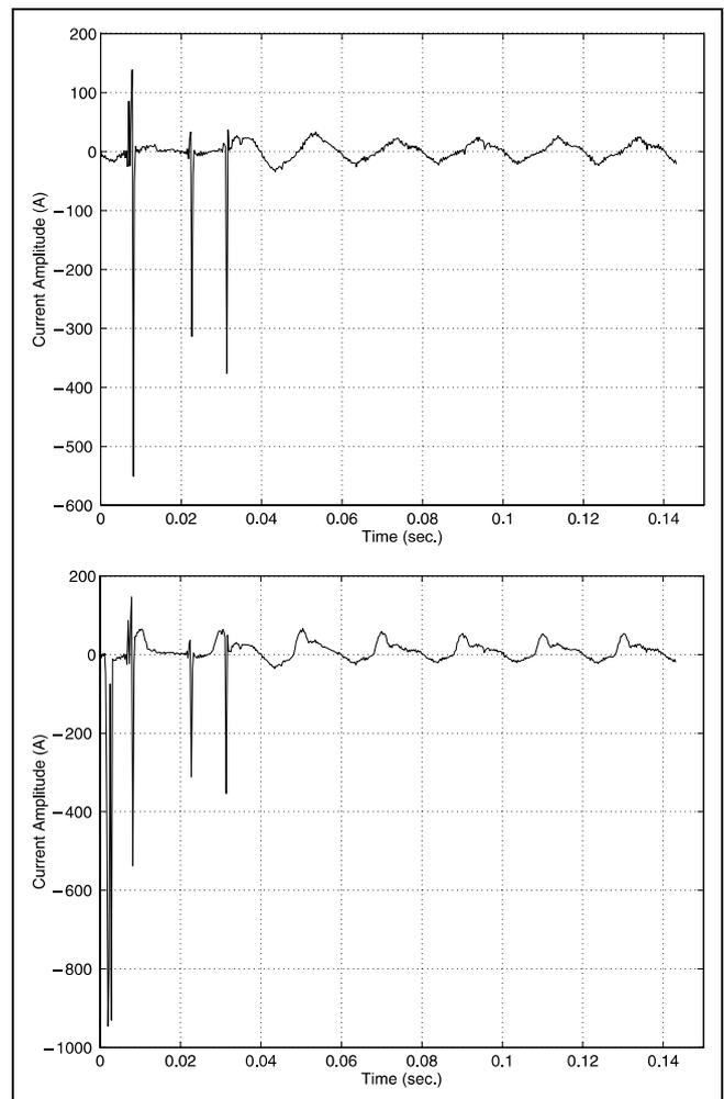
Figure 4: On the Top: Typical disturbance in the neutral section. On the Bottom: Inrush current and typical disturbance in superposition (the worst case).
