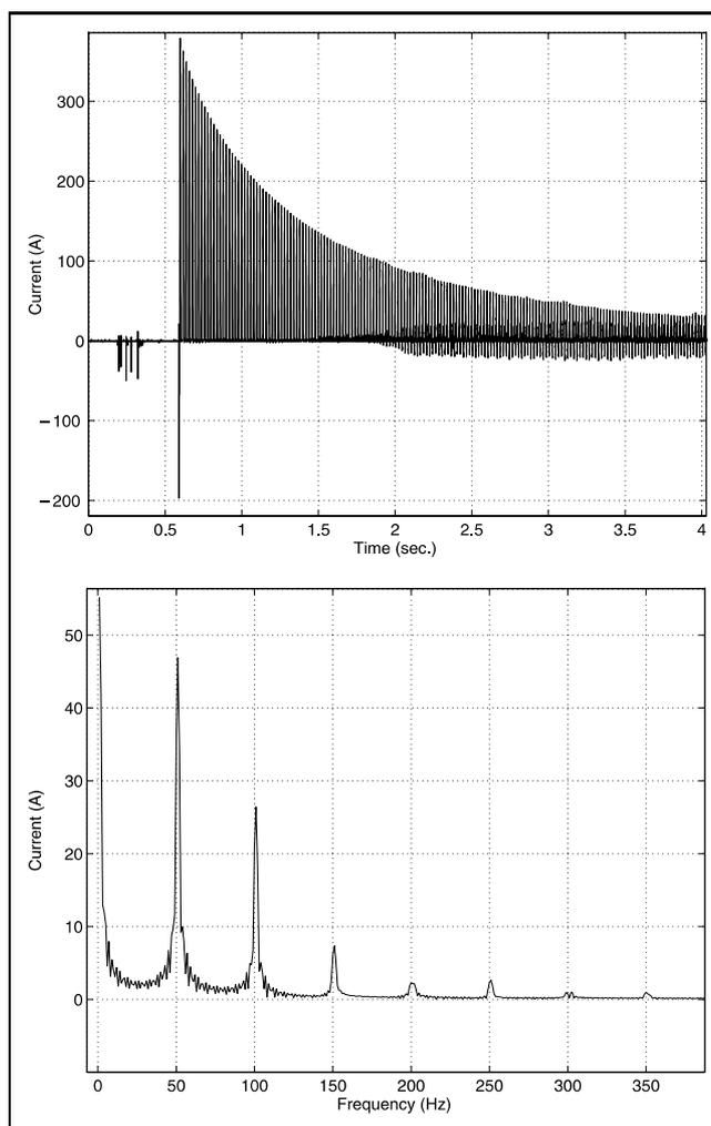
**Figure 2:** Real Signal. On the Top: Inrush current: time domain. On the Bottom: Inrush current: windowed spectral analysis.
