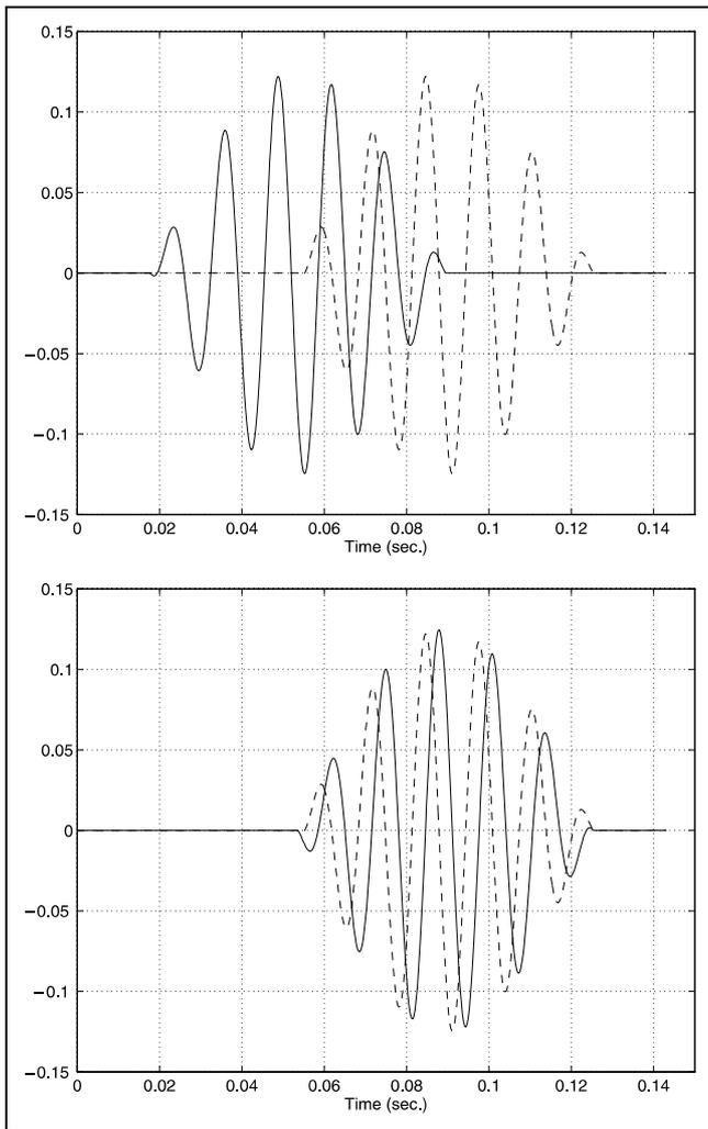
**Figure 1:** On the Top: Adjacent (orthogonal) cosine waveforms with smooth window  $C_{(2,1)}(t)$  and  $C_{(2,2)}(t)$ . On the bottom: biorthogonal smooth local sine and cosine function  $S_{(2,2)}(t)$  and  $C_{(2,2)}(t)$ .
