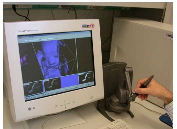
Figure 2. A) The 3D surface model of the fetus build from 2D ultrasound images and used for haptic visual interaction and the VR workstation comprising haptic and visual feedback. B) The hand moves the stylus of the Phantom desktop to touch the 3D VR model of the fetus.
