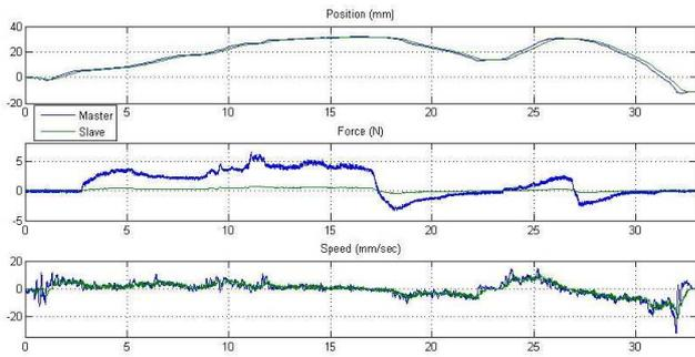
Fig. 14. Trajectories and energies for needle insertion using PD control.
