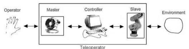
Fig. 1. The functional scheme of a teleoperator system.
