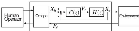
Fig. 5. The master-slave teleoperator system with the PD controller.
