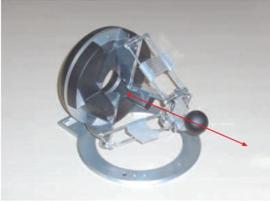
Fig. 2. The customized Omega.3 featuring a single translational DoF.
