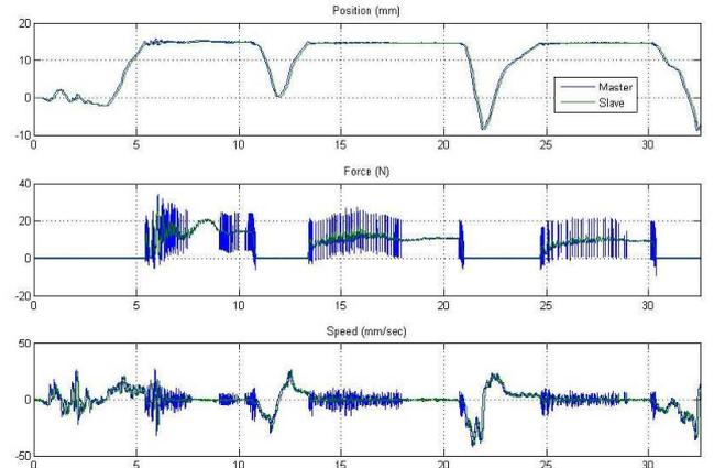
Fig. 7. Trajectories and energies for a rigid contact using PC control.
