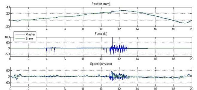
Fig. 13. Trajectories and energies for needle insertion using PC control.
