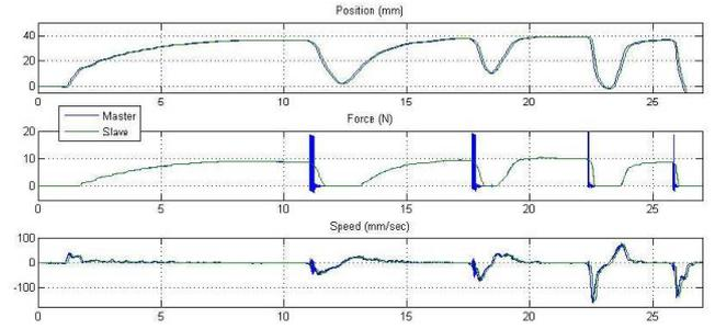
Fig. 10. Trajectories and energies for a soft contact using PC control.
