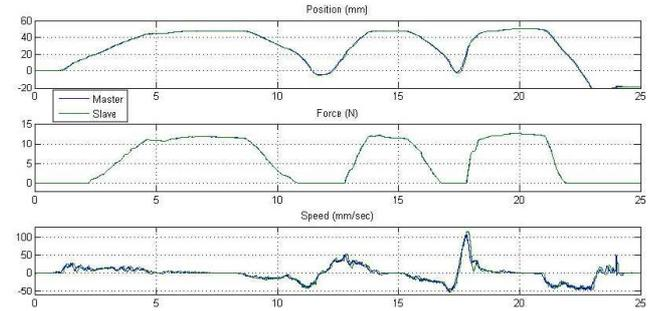
Fig. 11. Trajectories and energies for a soft contact using PD control.
