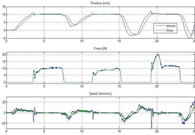
Fig. 8. Trajectories and energies for a rigid contact using PD control.
