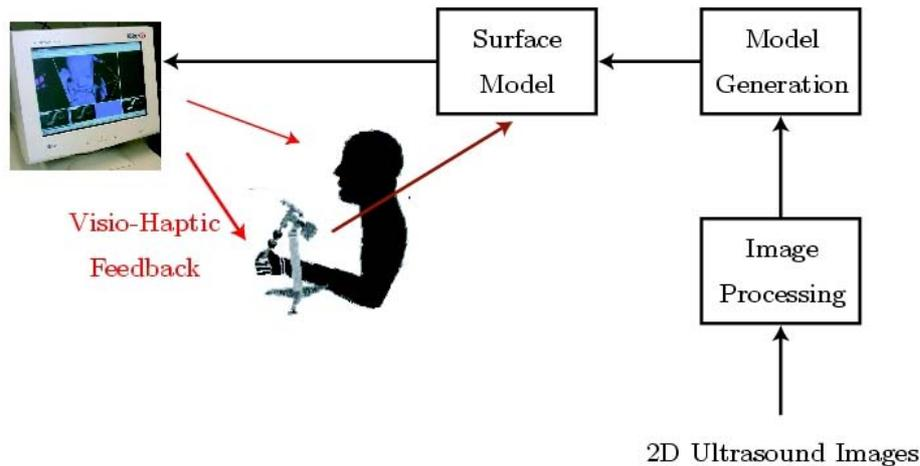
**Fig. 2.** The functional scheme of Fetouch .
