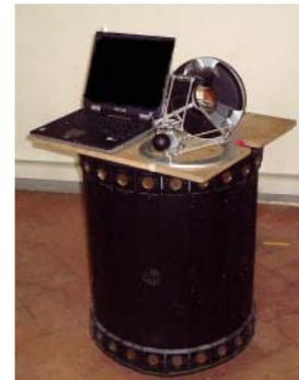
Figure 1: A prototype MHI combining an Omega Haptic Device with a Nomad XR4000 mobile platform.
