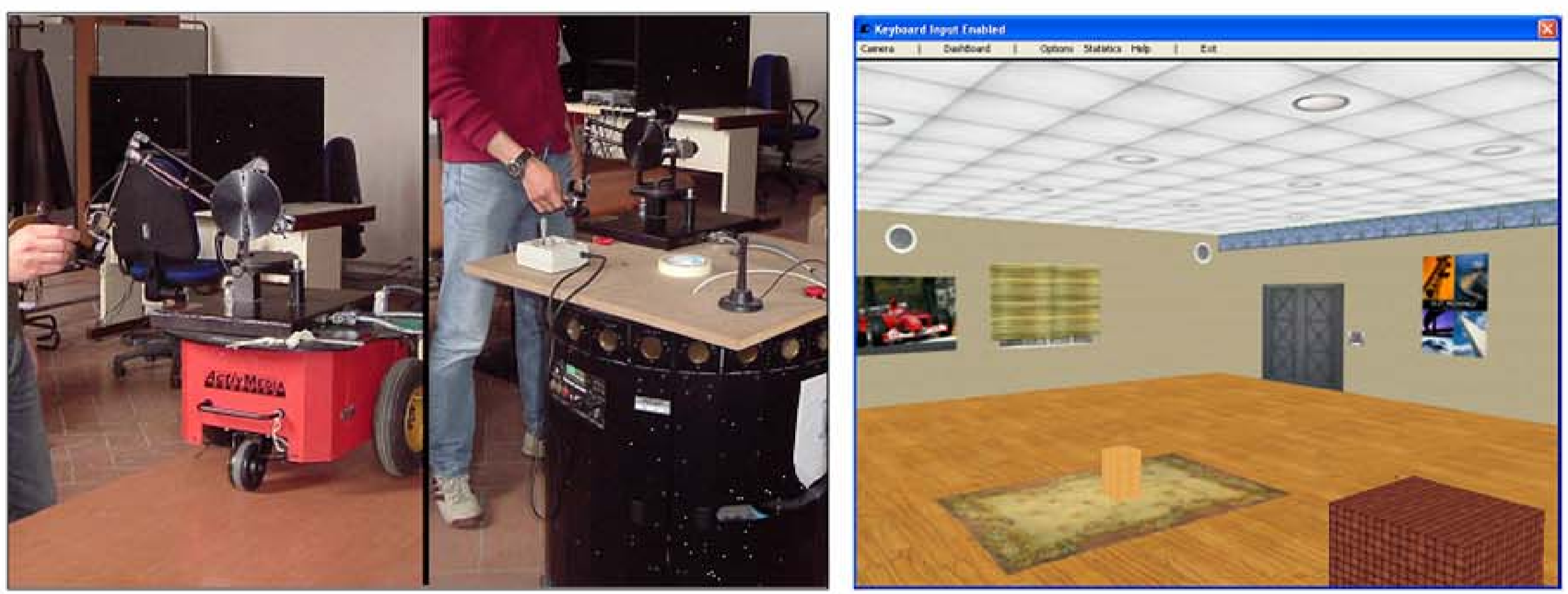
Two experimental MHIs: the PHANTOM with non-holonomic Pioneer2DX (left), and with holonomic Nomad XR4000 (right). Target environment: a virtual room
