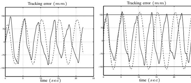
Fig. 7. Sine tracking errors of a mobile haptic interface realized with MP NomadXR4000. On the left, sinusoidal input is  $X_p(t) = 250 \sin(2\pi 0.2t)$ , on the right it is  $X_p(t) = 300 \sin(2\pi 0.2t)$ .
