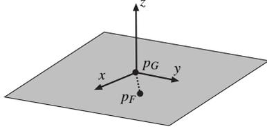
Figure 3: Local frame of reference associated with the contact surface.  $p_G$  and  $p_F$  denote the position of the god point and the position of the fingertip inside the object.
