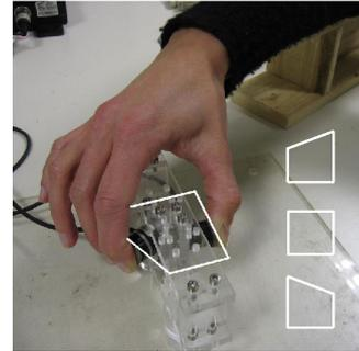
Figure 1: Experimental set-up used to measure finger forces in Experiment I (the screen hiding the view of the device to the subject is not shown). Inset: The three shapes shown at the end of the experiment.
