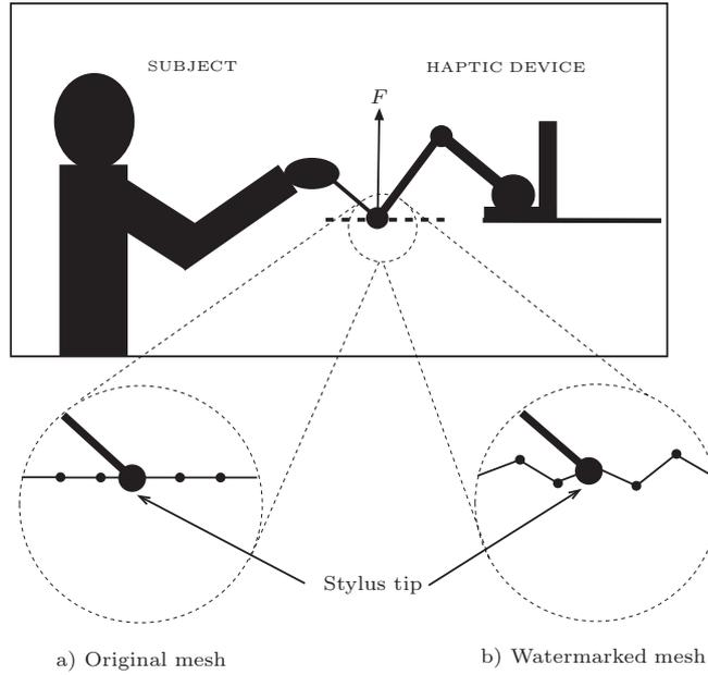
**Figure 3.** Haptic representation of the stimuli. (a) original mesh: all the vertices lay on a plane. (b) watermarked mesh: vertices heights are altered by the watermark.
