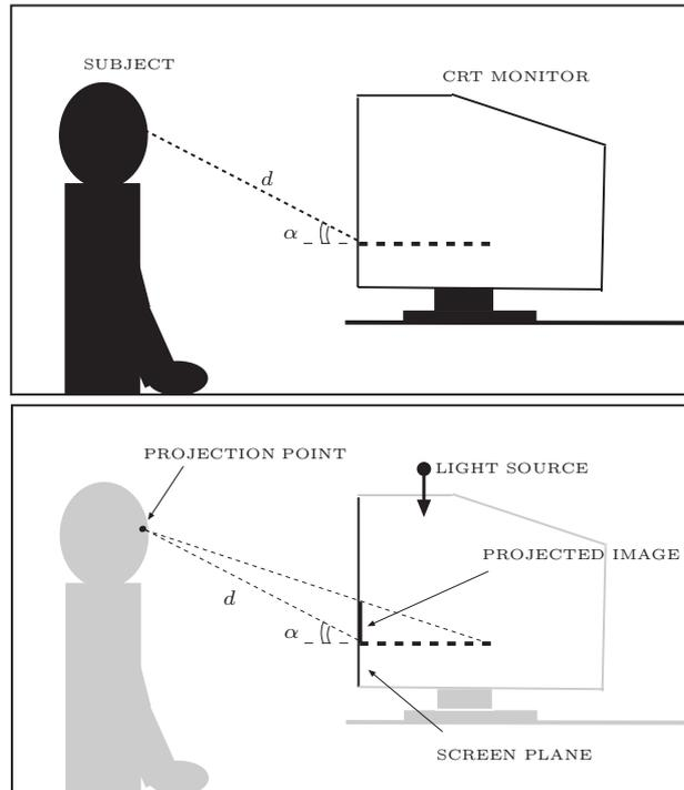
**Figure 5.** Geometrical set up for the visual stimuli. Top: user's displacement w.r.t. monitor. Bottom: rendering conditions.
