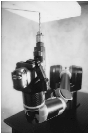
Figure 2: The Barrett Hand mounted on a host arm grasping an electric drill. The hand is a multi-fingered programmable grasper with the dexterity to secure target objects of different sizes, shapes, and orientations. The hand has a low weight (1.18kg) and compact form. ( Courtesy of Barrett Technology Inc. )
