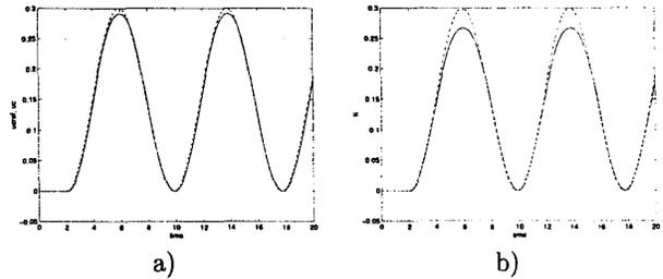
**Figure 5:** Rigid–body object motions starting from the initial configuration in fig. 4. (a) Logic–based switching control: reference input  $\mathbf{u}_{c,ref}$  (dash-dotted line) and system output  $\mathbf{u}_c$ . (b) Linearized control: reference input  $\mathbf{u}_{c,ref}$  (dash-dotted line) and system output  $\mathbf{u}_c$ .
