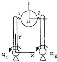
**Figure 4:** Simple 2-joints, 2-contacts 2D general manipulation system. In this configuration,  $q_1 = q_2 = 0$ ,  $\mathbf{u} = [\mathbf{u}_x, \mathbf{u}_y, \theta]^T = [1.5, 3, 0]^T$ .
