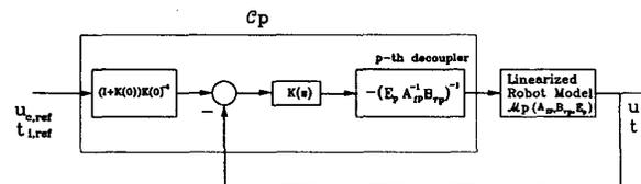
**Figure 1:** Asymptotic reproducible controller  $\mathcal{C}_p$  for linearized model  $\mathcal{M}_p$ .
