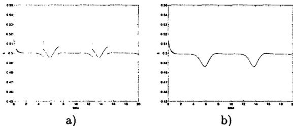
**Figure 6:** Reachable internal force behaviour when the reference input is a step of 0.5N. To the initial configuration (fig. 4), It corresponds a zero internal force. (a) Logic-based switching. (b) Linearized control with  $\sigma = 1$ .
