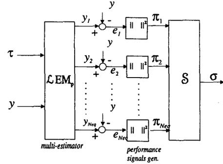
**Figure 3:** Multiestimator based supervisor.
