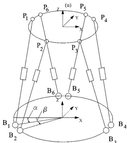
Fig. 8. The model of a 6-DOF Stewart platform.
