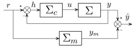
Fig. 13. Model following with feedback.
