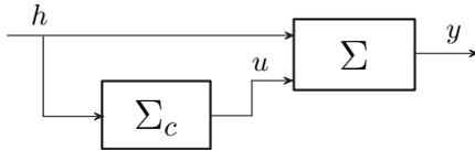
Fig. 5. Measurable signal decoupling with a feedforward compensator.
