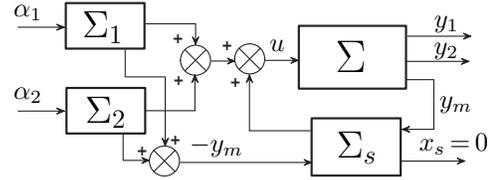
Fig. 17. Using a stabilizer in feedforward noninteracting control.
