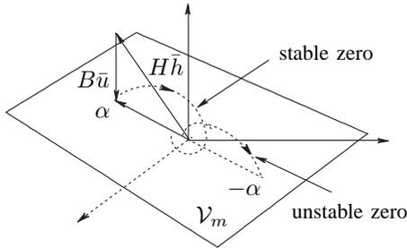
Fig. 10. Preaction along the unstable zeros.
