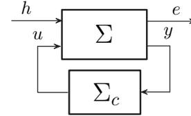
Fig. 11. Disturbance decoupling by dynamic output feedback.
