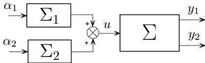
Fig. 16. Noninteracting control with dynamic feedforward units.
