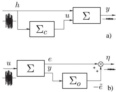
Fig. 21. (a) Kalman dual filter; (b) Kalman filter.
