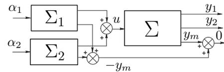
Fig. 18. Nulling a measurable output.
