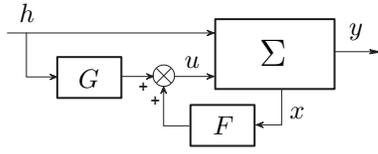
Fig. 4. Measurable signal decoupling with state feedback.
