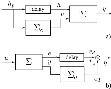
Fig. 9. (a) Previewed decoupling; (b) Delayed unknown-input observation.
