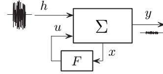
Fig. 20. Minimal  $H_2$ -norm decoupling (Kalman regulator).
