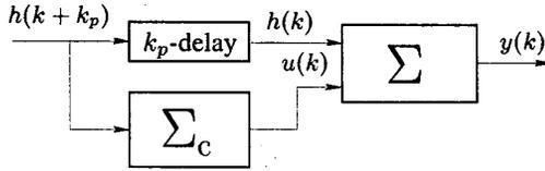
**Figure 1:** Decoupling of a measurable or previewed signal.
