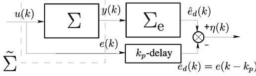
Fig. 4. Block diagram for stable left inversion with fixed lag.
