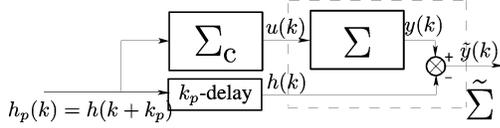
Fig. 3. Block diagram for stable right inversion with preview.
