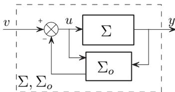
Fig. 2. Using a stabilizer.
