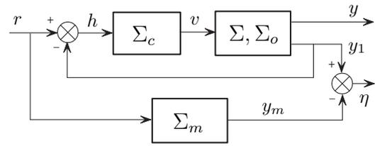
Fig. 6. Modified feedback model following.
