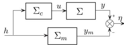
Fig. 1. Feedforward model following.
