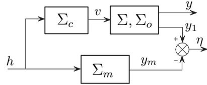
Fig. 4. Modified feedforward model following.
