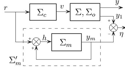
Fig. 8. Block diagram for the equivalent feedforward model following.
