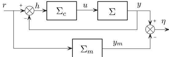
Fig. 5. Exact feedback model following.
