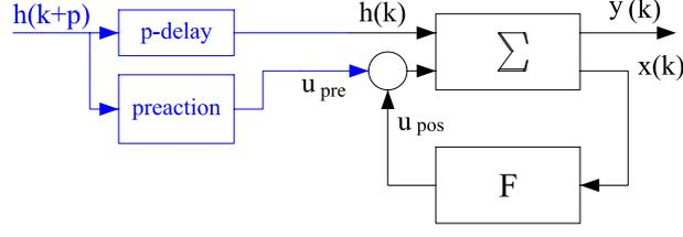
Figure 2: The decoupling compensator consists of a preaction unit and a postaction unit.
