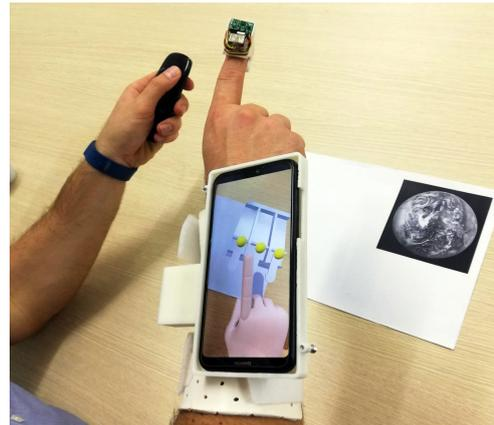
Fig. 1: The haptic device worn on the fingertip together with the wrist-worn display for MAR. In this picture the left hand is free and holds a remote controller.
