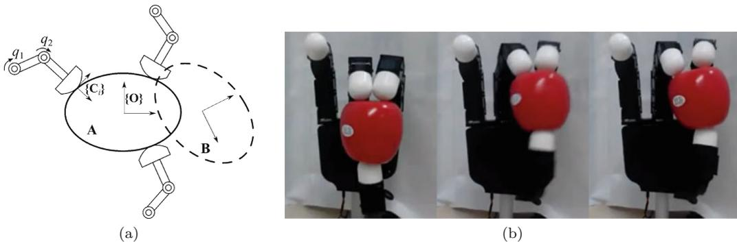
**Dexterous Manipulation, Fig. 1** (a) Dexterous manipulation problem definition: moving an object from configuration **A** to configuration **B**,  $\{O\}$  is the object coordinate
