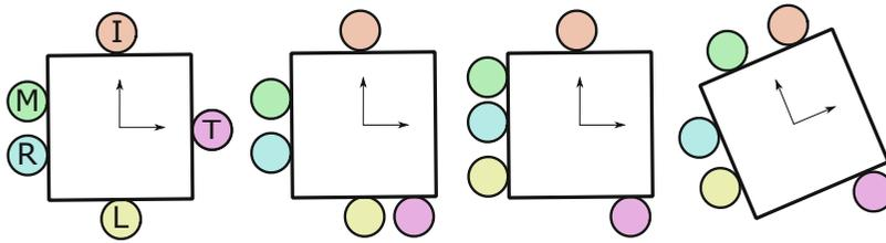
**Dexterous Manipulation, Fig. 3** Sketch of a dexterous manipulation using finger relocation performed by an anthropomorphic hand with thumb (T), index (I), middle (M), ring (R), and little (L) fingers
