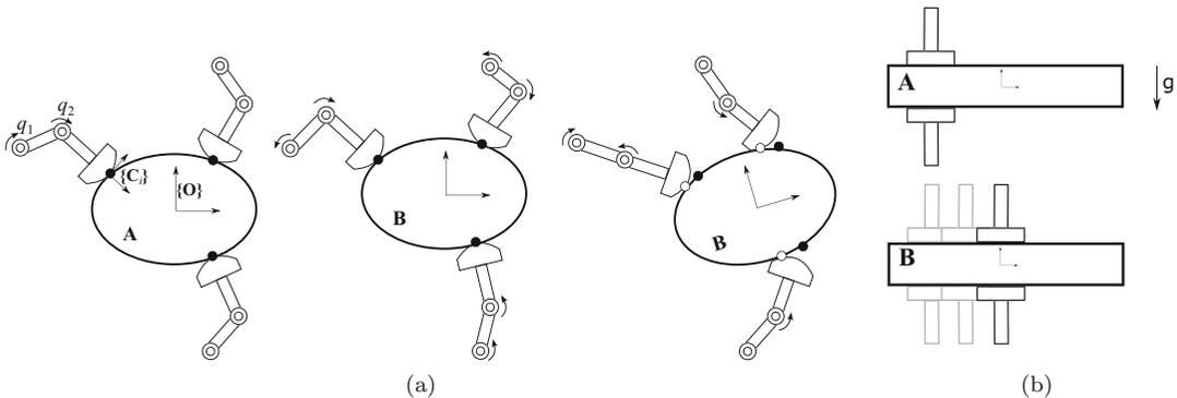
**Dexterous Manipulation, Fig. 2** (a) (left) Initial grasp configuration, (middle) final configuration obtained through a coordinated motion of the fingers without moving the initial contact points depicted in black, and (right) final configuration obtained by explicitly using contact rolling, generating the new contact point locations
