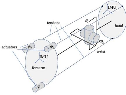
Fig. 2: Wrist and exoskeleton scheme. The wrist is modelled as a 2 DoFs universal joint, enabling the flexion/extension  $\theta_e$  and adduction/abduction  $\theta_a$  of the hand w.r.t. the forearm. Three tendons connect the exoskeleton hand and forearm supports and are actuated with three motors. Their angular rotation is indicated with  $\phi_i$ .
