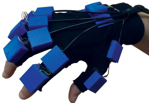
Fig. 1: The glove is made by 11 MARG boards (blue) for sensing. It allows to estimate the joints values and rotation of the human hand with respect to a global reference frame. The last phalanx of each finger is left uncovered to not affect the user's tactile perception.
