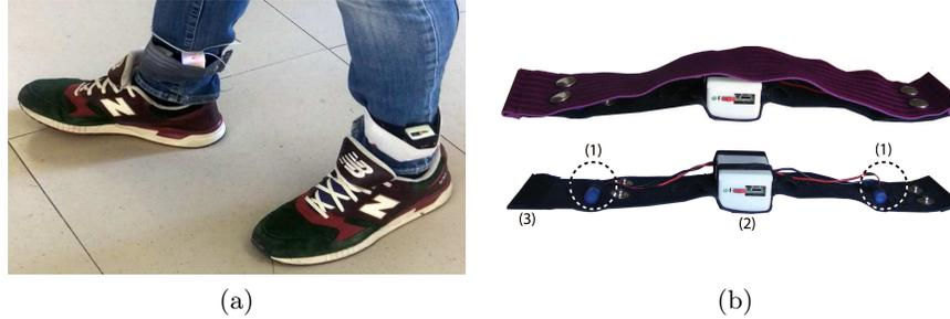
Fig. 2: Cadence cues are provided to the users via two vibro-tactile elastic bands placed on the ankles (a). The haptic bands (b) are composed of two vibrating motors (1) attached to an elastic wristband (3). A Li-Ion battery is in charge of power and an Arduino board controls the interface (2).
