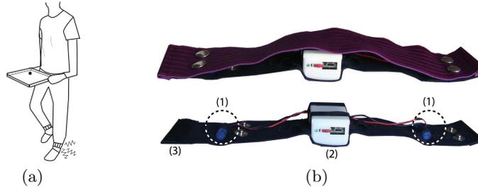
**Fig. 1.** Cadence cues are provided to the users via two vibro-tactile elastic bands placed on the wrists or on the ankles (a) of the user during a task with manual and cognitive load. The haptic bands (b) are composed of two vibrating motors (1) attached to an elastic wristband (3). A Li-Ion battery is in charge of power and an Arduino board controls the interface (2).
