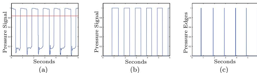
**Fig. 2.** The pressure values are recorded by a flexible force sensor (FSR 400) and sent wireless through a XBee radio module. The raw signal showed in (a) is normalized between 0 and 1. Steps are extracted by thresholding the raw signal (b), and only considering the positive edges (c). The threshold is set at  $2*STD$  (Standard Deviation).
