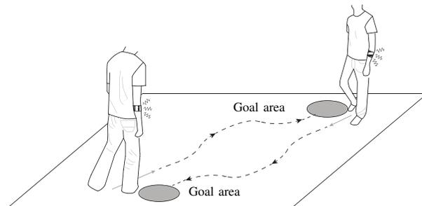
Fig. 1. We address the problem of guiding human subjects in situations with poor/no visibility. The subjects have to reach the respective goal areas while avoiding collisions with static obstacles and moving users. Each user wears two vibrotactile armbands which provide appropriate directional cues.
