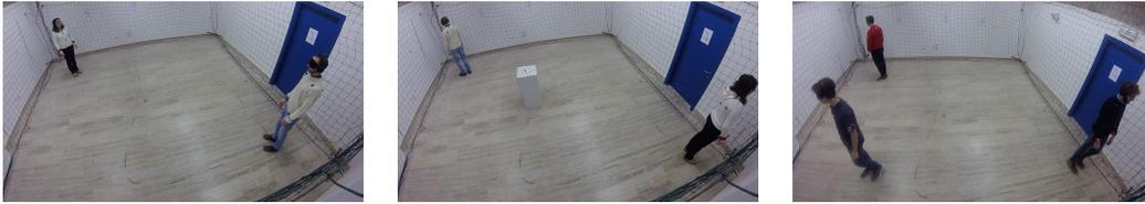
Fig. 2. Experimental validation for all three scenarios. The blindfolded and audio-occluded users have to move towards their goal areas by following directional cues provided by haptic armbands. (Left) Scenario with only two users; (Center) Scenario with two users plus an obstacle; (Right) Scenario with three users.
