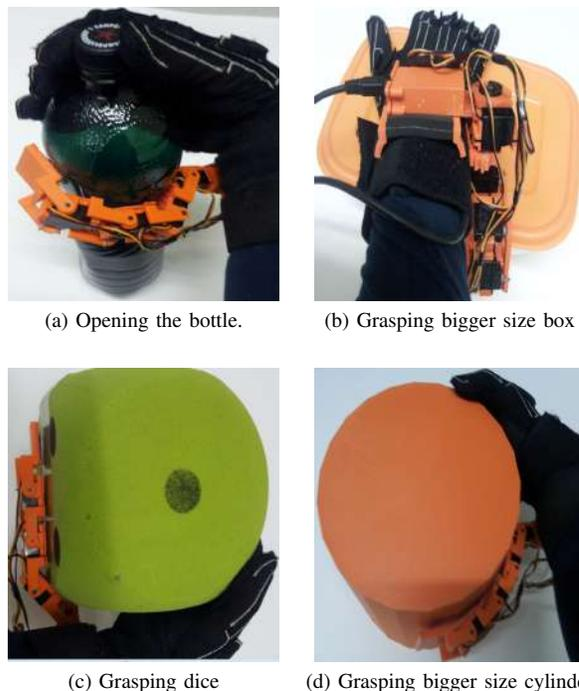
Fig. 3. Examples of tasks performed during the training with the supernumerary robotic finger.
