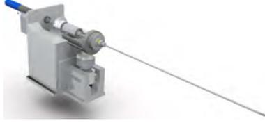
Fig. 6. 2-DoF motorized microsurgical forceps assembled with actuator housing
