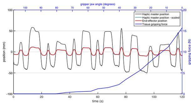
Fig. 7. Motion control and tissue gripping force evaluation
