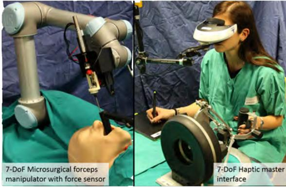
Fig. 2. Robot-assisted microsurgical forceps concept
