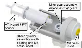
Fig. 5. Mechanism housing
