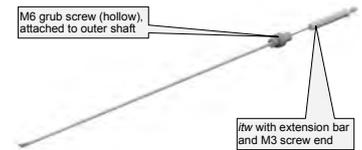
Fig. 4. Main tool shaft - adaptations
