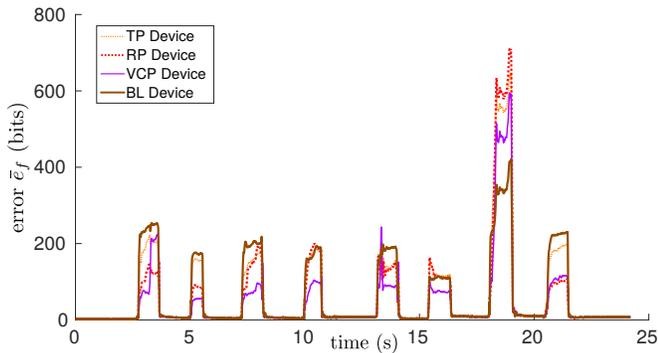
Fig. 6. Experimental evaluation. Error  $\bar{e}_f$  registered during a representative interaction with the Medium material. At each time step, each cutaneous device attempts to present the tactile sensations measured while the BioTac pinched the material.
