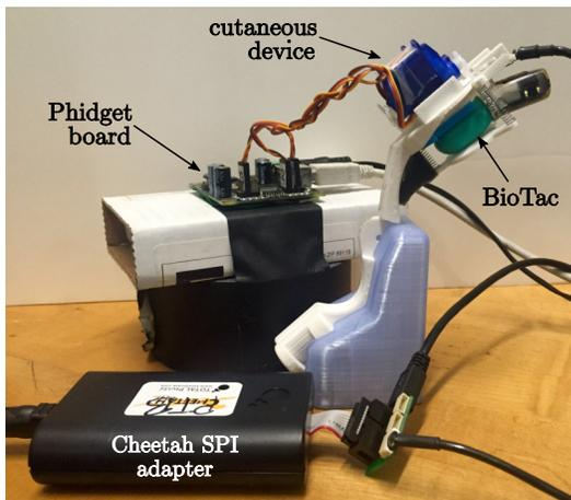
Fig. 2. Calibration setup featuring the BioTac mounted in the rigid plate cutaneous display. The BioTac is connected to the computer through a Cheetah high-speed SPI adaptor, and the servo motors are controlled through a Phidget servo board.
