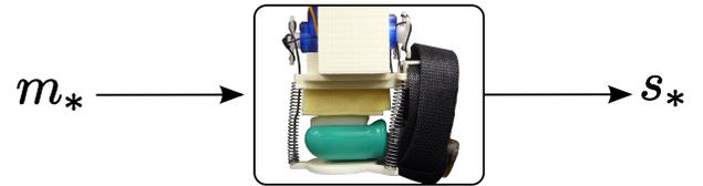
Fig. 2. Data collection. The BioTac was placed inside the cutaneous device, and the platform was moved to a wide range of configurations. The motor inputs  $\mathbf{m}_*$  and the resultant cutaneous sensations  $\mathbf{s}_*$  were recorded.
