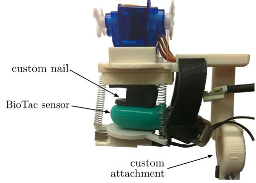
Fig. 4. Data collection. The BioTac was placed inside the cutaneous feedback device, and the platform was moved to 39304 different configurations. Servo motor inputs  $m_{d,*}$  and the resulting effect on the tactile sensor's electrodes and DC pressure  $s_{d,*}$  were recorded. For 4913 of these configurations, we also played a two-second-long swept sine wave (1 Hz – 1000 Hz) through the vibrotactile motor and registered its effect on the BioTac's pressure sensor  $s_{v,*}$  (AC signals).
