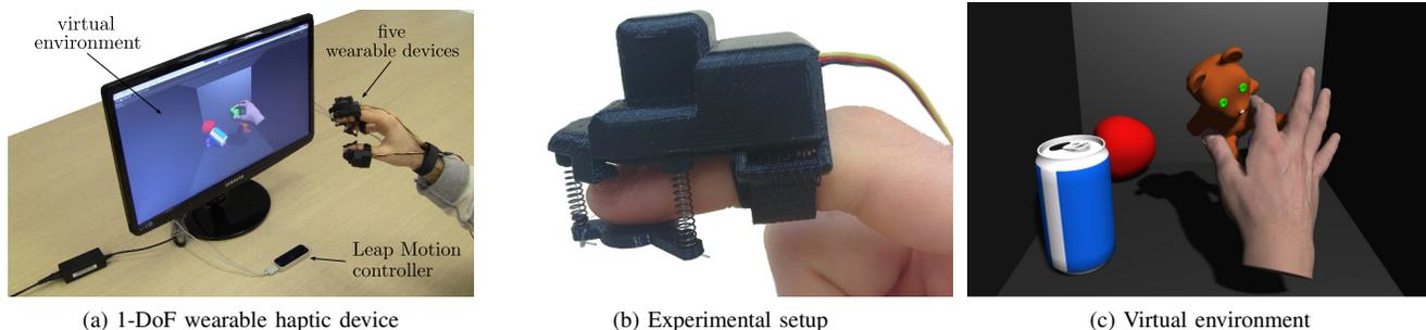
Fig. 1. Immersive tactile interaction in a virtual environment. User's fingertips are tracked using a Leap Motion controller (a) while five wearable tactile interfaces (b) provide the human operator with the compelling illusion of touching a virtual object (c).
