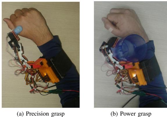
Fig. 3. The two predefined flexion paths for the robotic extra finger. In (a) the grasp is obtained between the fingertip of the device and the thenar eminence. In (b) the grasp involve the whole device and the user wrist.
