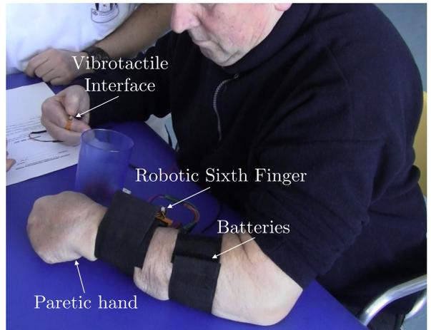
Fig. 1. The robotic extra finger together with the vibrotactile interface ring. The ring provides haptic feedback through a vibrating motor and enable the user to start and stop the finger motion through a switch.
