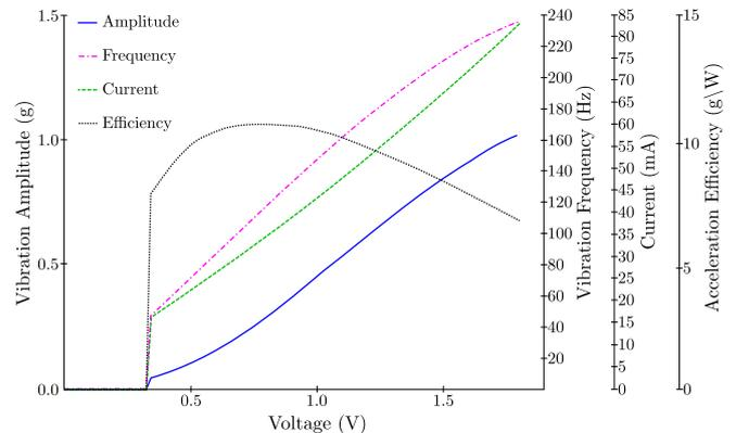
Fig. 4. Typical performance characteristics of the Precision Microdrives 4 mm Vibration Motor (11 mm type).
