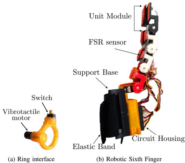
Fig. 2. CAD models of the vibrotactile interface and of the modular finger. Four modules are connected to a wrist elastic band. The ring is equipped with a push button used as an interface with the user and a vibrotactile motor to provide an haptic stimulus.
