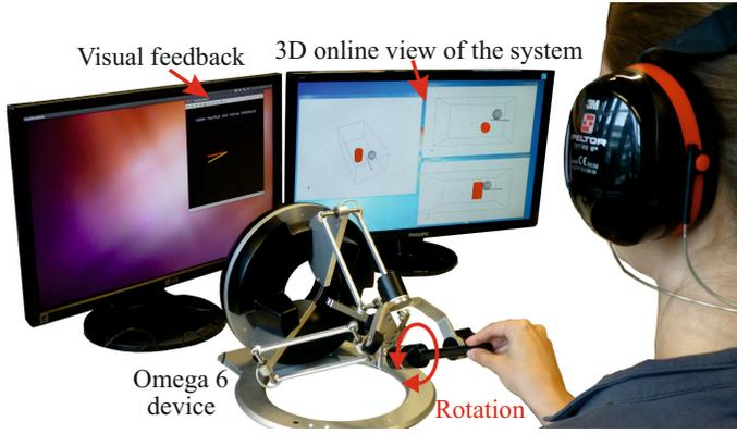
Fig. 4. Experimental evaluation. The subject performs an experimental trial while receiving both visual and vibratory feedback (VI+VB). The subject is asked to follow the online three-dimensional (3D) view of the system on the right screen and the visual feedback on the left screen.
