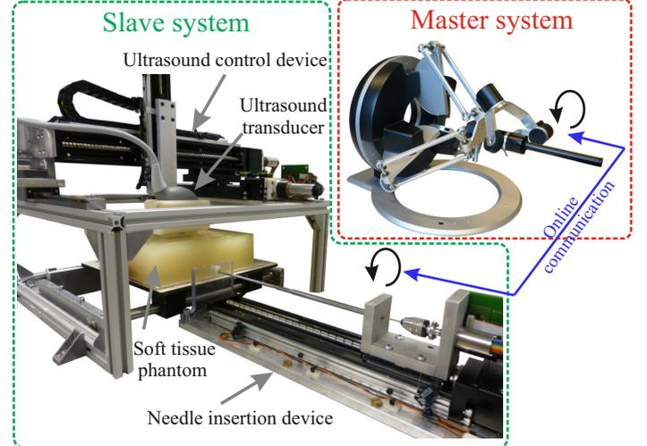
Fig. 1. The slave system represents the needle control device for needle insertion and rotation about its axis, and also the ultrasound control device used for three-dimensional needle tip tracking. The master device represents the haptic device that allows the operator to control the needle.
