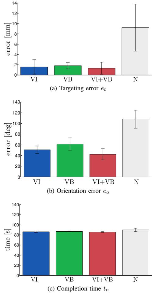
Fig. 5. Needle insertion experiment. Targeting error  $e_t$ , orientation error  $e_o$ , and completion time  $t_c$  (mean and SD) are plotted for the experimental conditions where the subjects receive visual (VI), vibratory (VB), visual and vibratory (VI+VB), and no (N) feedback from the control algorithm. Lower values of this metrics indicate higher performances in completing the given task.
