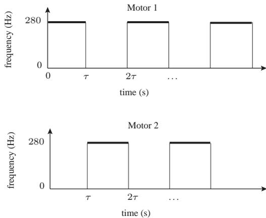
Fig. 2. In order to keep signal recognition as simple as possible, the two motors of the bracelet vibrate alternately with period  $2\tau$ .
