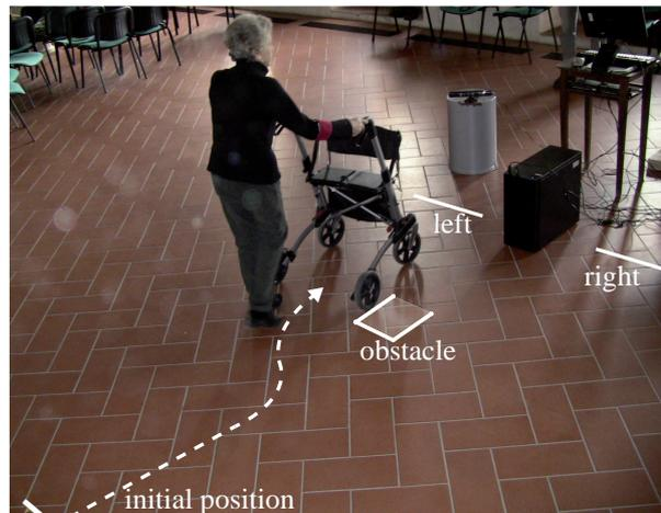
Fig. 3. The user had to avoid the obstacle by turning left or right, depending on the vibrating stimuli.
