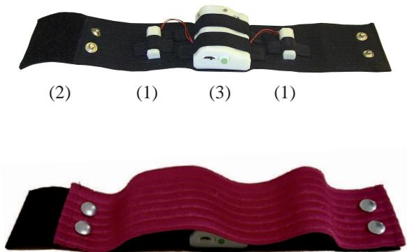
Fig. 1. The vibrotactile bracelet equipped with two vibrating motors (1) attached to an elastic wristband (2). The Li-Ion battery and the Arduino board are in (3).
