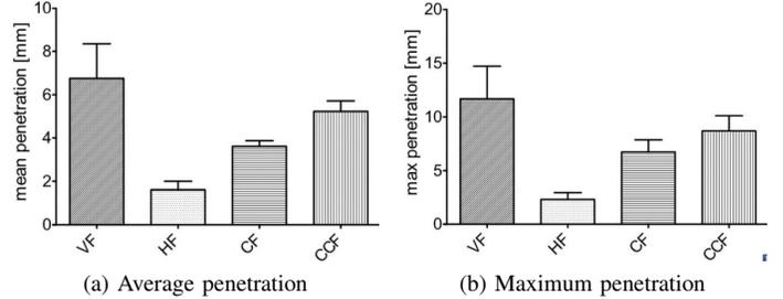
Fig. 3: Experiment of sensory subtraction in [1]. Average and maximum penetration beyond the stiff constraint (mean and std), for the visual (VF), haptic (HF) and cutaneous feedback conditions (CF, CCF). A null value of this metric indicated the best accuracy in reaching the target depth. The sensory subtraction approach is employed in condition CF.
