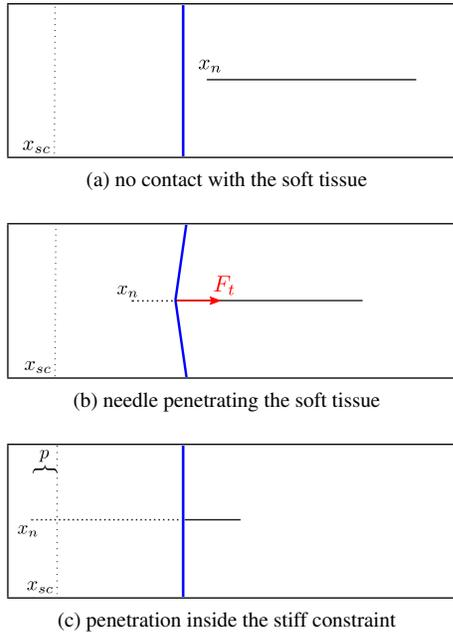
Figure 3: The virtual environment was composed of the needle (black), driven by the operator, the deformable tissue (blue), and the stiff constraint (red). The position of the needle  $x_n$  was linked to the position of the haptic device end-effector, the position of the stiff constraint was fixed to  $x_{sc}$ , and  $p$  represented the penetration of the needle inside the stiff constraint. Dashed parts were not visible by the subjects.
