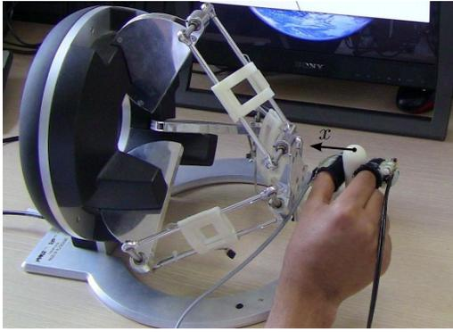
Figure 2: Experimental setup. The users were asked to wear two cutaneous devices, one on the thumb and one on the index finger, and grasp the handle with their right hand, positioned with its longitudinal axis at 90 deg from the Omega  $x$ -axis.
