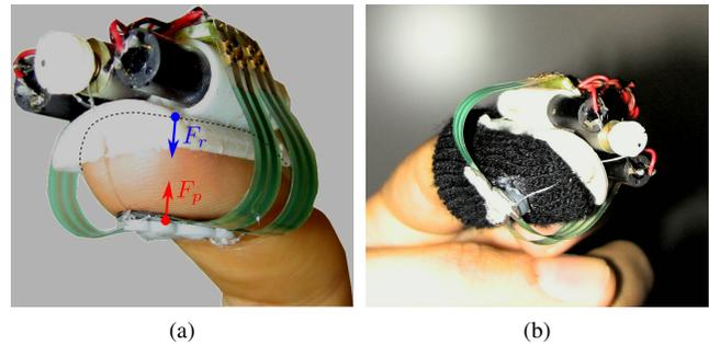
Figure 1: The 3-DoFs wearable haptic display. The motors, acting on the lengths of the three wires, provide the requested force  $F_p$  to the user's fingertip (red arrow). This force is balanced by another one,  $F_r$ , supported by the structure of the device on the back of the finger (blue arrow).
