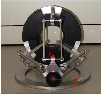
Figure 2: Experimental setup. The Omega 3 single-contact haptic device has been used in the experiments to provide vibrotactile and kinesthetic force feedback. The figure shows the  $y$  and  $z$  axes of the display.
