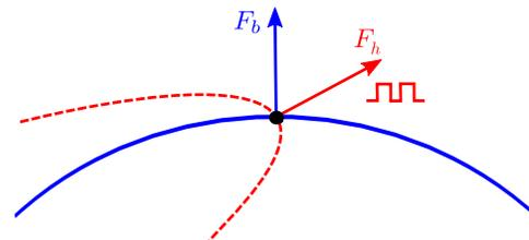
Figure 1: Proposed scenario, mixing kinesthetic and vibrotactile force feedback. The end-effector is shown in black, a remote object and resulting contact force ( $F_b$ ) in blue, a virtual fixture and resulting vibrotactile force feedback ( $F_h$ ) in red.
