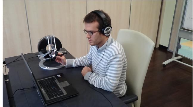
Figure 1: The experimental setup: the user moves his hand along a line, the haptic device is constrained on, and retracts as he perceives an alert which can be a vibratory, visual or auditory cue.
