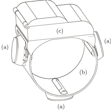
**Figure 3:** The human-robot interaction is achieved via a vibrotactile bracelet equipped with three vibrating motors (a): *L* (left), *C* (center) and *R* (right) attached to an elastic strap (b). The three motors are disposed equidistantly in order to improve the vibrotactile perception. A 9V battery and an Arduino board are disposed on the back of the forearm (c).
