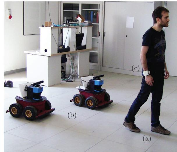
Figure 1: A human leader (a) is followed by a team of mobile robots (b) equipped with RGB-D cameras. A vibrotactile bracelet (c) allows the followers to inform the leader about the formation consistency.
