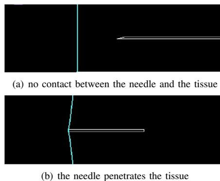
Fig. 4. The virtual environment is composed of the needle (white), driven by the operator, the deformable tissue (cyan), and the stiff constraint. The position of the needle in the virtual environment is linked to the position of the haptic device end-effector.
