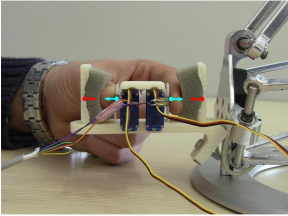
Fig. 2. The cutaneous device mounted on the Omega 3 end-effector. The motors flex the platforms, applying a force to the thumb or to the index finger (cyan arrows). Each force is balanced by a force supported by the structure of the device on the back of the each finger (red arrows).
