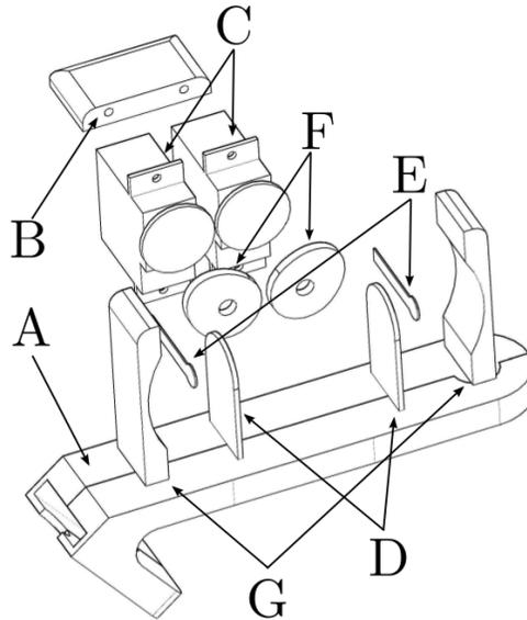
Fig. 1. CAD rendering of the handle prototype. Part A is fixed to the haptic device end-effector while parts B and F permit to use the torque of the motors (C) to flex the two platforms (D). Two sensors (E) are in charge of registering the actual force applied by the device while platforms G support the fingers.
