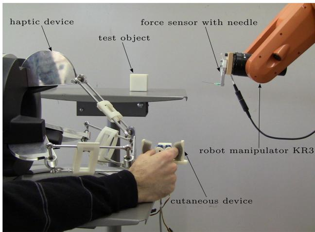
Fig. 10. The experimental setup. The haptic device, with the proposed device mounted on, controls the motion of the manipulator. The force measured at the needle tip by a sensor is fed back to the operator either by the motors of the Omega 3 or by the motors of the cutaneous device.
