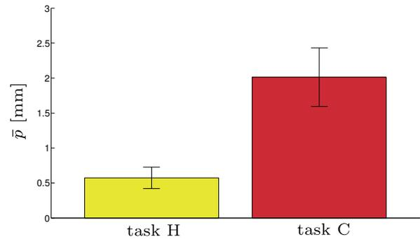
Fig. 7. Experiment in a simulated environment. Mean penetration depth  $\bar{p}$  into the stiff constraint, expressed in [mm], during tests with the haptic (task H) and cutaneous feedback (task C).
