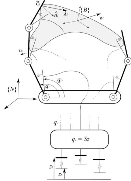
Fig. 2. The soft synergy actuated hand, from [16].
