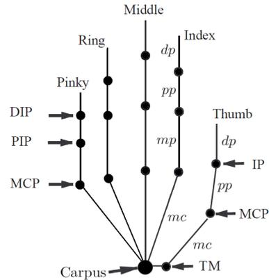
Fig. 3. Scheme of the *paradigmatic* hand highlighting the joints and the links.
