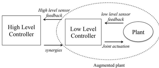
Fig. 6. Two stage controller for a robotic hand: the high level stage is low dimensional and independent from the controlled device, the low level transforms the synergy inputs into joint reference values.
