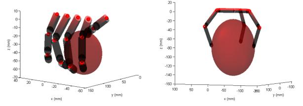
Fig. 4. The human-like hand (left) and the robotic hand (right) grasping a sphere with three contacts.
