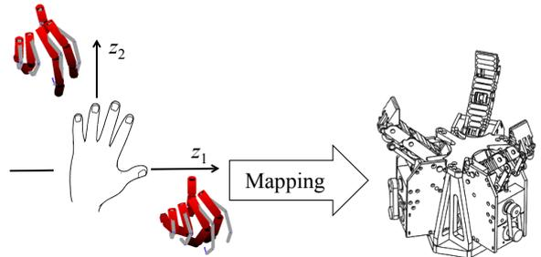
Fig. 1. Mapping between human synergies and robotic hands.
