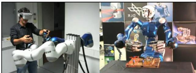
Fig. 1. Example of a teleoperation system where the user teleoperates by the remote robot. Courtesy of Institute of Robotics and Mechatronics German Aerospace Center (DLR),
