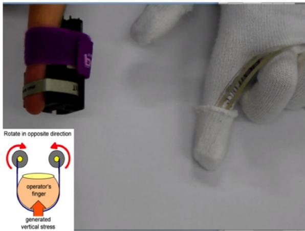
Fig. 3. The glove instrumented with force sensors on the right and the tactile display (with the functional scheme) on the left.
