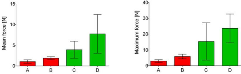
**Fig. 2.** Mean (left) and maximum (right) contact forces, expressed in [N], during tasks A, B, C ad D. Each bar represents the average of all participants for a single task. Red bars indicate kinesthetic feedback, green bars indicate tactile feedback.
