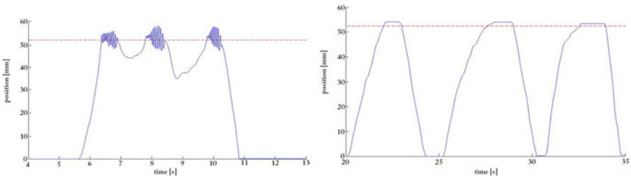
**Fig. 3.** Joystick probe position  $x_h(t)$  expressed in [mm] using kinesthetic feedback (left) and tactile feedback (right), with a network delay of 0.1s in the haptic loop. Dotted red lines represent the position of the virtual wall.
